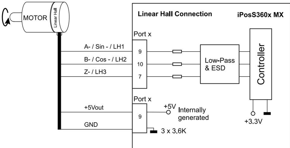
5.7 Connecting an analog encoder (sine-cosine)
